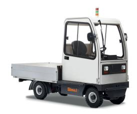
4-wheel platform truck, man on board, with rear-wheel drive. Extremely compact and easy to drive, ideal for all duties - both indoors and outdoors, even on long distances. The platform of the PE15 truck can be completed with other equipment.
