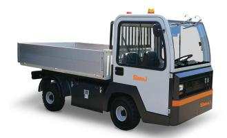
4-wheel platform truck, man on board, with rear-wheel drive. Extremely easy to drive, ideal for all duties - both indoors and outdoors, even on long distances. The platform of the PE30 truck can be completed with other equipment.
