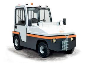
4-wheel tow tractor, man on board. Heavy-duty high-performance and long-range truck for industrial and airport duties. Despite its small size and turning radius, the TE300R has a high towing capacity. Driving position is located backwards ensuring optimum weight distribution and excellent stability. Loading capacity of front platform 80 kg.
