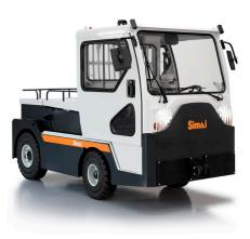
4-wheel tow tractor, with on-board operator. Heavy-duty high-performance and long-range truck for industrial and airport duties. Despite its small size and turning radius, the **TE252** has a 25-tonne towing capacity. **TE293** version with 29-tonne towing capacity. Loading capacity of wide rear platform 200 kg.
