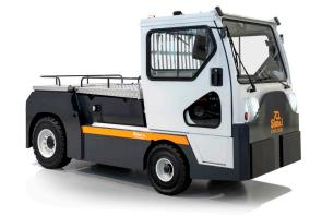
4-wheel tow tractor, with on-board operator. Heavy-duty high-performance and long-range truck for industrial and airport duties. Despite its small size and turning radius, the TE501 has a 50-tonne towing capacity. Loading capacity of wide rear platform 200 kg.
