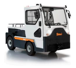
4-wheel tow tractor, with on-board operator. Heavy-duty high-performance and long-range truck for industrial and airport duties. Despite its small size and turning radius, the **TE293** has a 29-tonne towing capacity.
