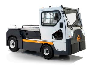
4-wheel tow tractor, with on-board operator. Heavy-duty high-performance and long-range truck for industrial and airport duties. Despite its small size and turning radius, the TE501 has a 50-tonne towing capacity. Loading capacity of wide rear platform 200 kg.
