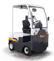
4-wheel tow tractor, man on board, with rear-wheel drive. Extremely compact and easy to drive, ideal for all industrial duties - both indoors and outdoors, even on long distances.
