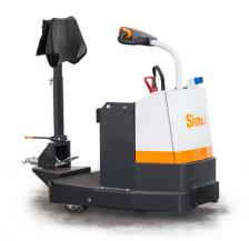
3-wheel tow tractor, man on board, with front-wheel drive. Extremely fast, compact and easy to drive, perfect for indoor lightweight, short-distance, industrial towing duties.
