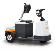
3-wheel tow tractor, man on board, with rear-wheel drive. Extremely compact and easy to drive, ideal for LEAN handling duties.
