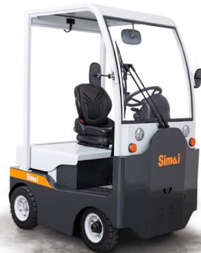
4-wheel tow tractor, man on board, with rear-wheel drive. Extremely compact and easy to drive, ideal for all industrial duties - both indoors and outdoors, even on long distances.
